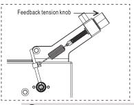
Rotate the feedback tension knob to adjust the back tension. Clockwise: Back tension increases Anti-clockwise: Back tension decreases
