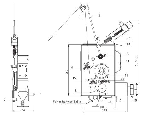
The round thread 2 Tension rod 3 Tension rod fixing seat 4 Wire jump 5 The wool felt regulator knob
